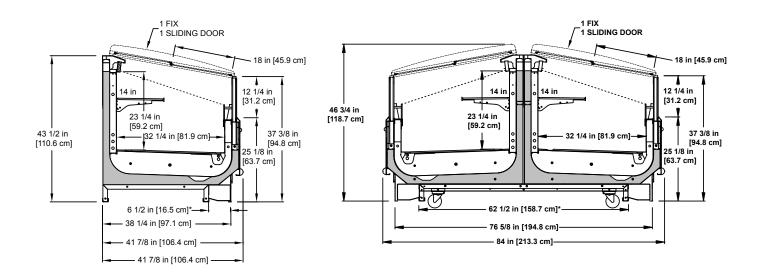
Please consult Hillphoenix Engineering Reference Manual for dimensions, plan views and technical specifications. Specifications subject to change without notice. Designed for optimal performance in store environments where temperature and humidity do not exceed 75°F and 55% R.H. Certified to UL 471 and ANSI/NSF Standard 7.
